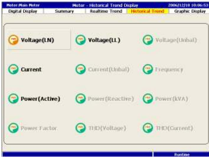
Similar to real time trend, PM1600 can display various power data for each meter. The display items are the same as real time trend which are pre determined in the configuration mode for each meter.
